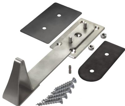
Stable shear retainer, made of solid stainless steel, to be installed on sealed pitched roofs as loose flange / fixed flange construction. Replaces wooden shear barriers in connection with ZinCo eaves profiles.
