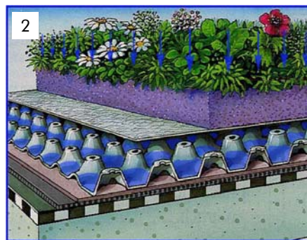
Excess water moves downwards through the filter sheet into the drainage element where a significant amount of water is stored.
