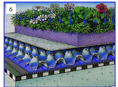
Any excess water that cannot be stored by the system build-up is drained away quickly and securely.
