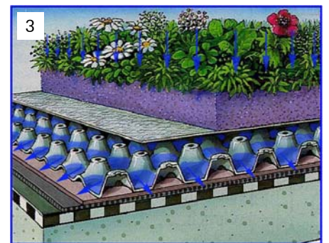
Excess water overflows the cups and through the joints of the drainage element reaches the canal system underneath.
