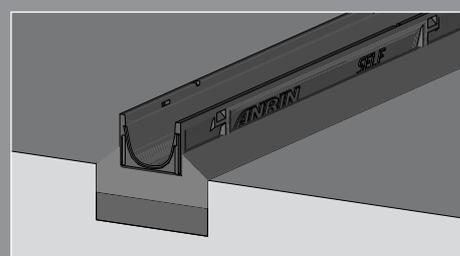
Connect pipe connections to the pipeline and align the components evenly. Fill concrete bed.
