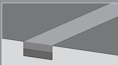
Form concrete bed, 3 parts sand + 1 part water + 1 part cement, on base course.
