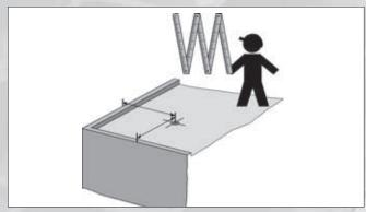
1. Measuring the position of the anchor point
